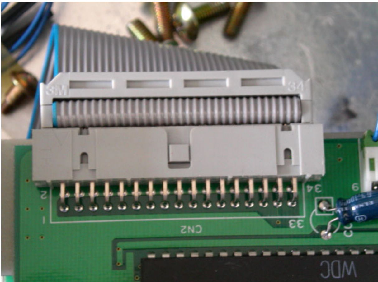
Picture1: The 34-pin connector of the floppy controller of an EL90 organ.
